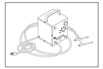
Figure 7. One Type of Hi-Pot Tester
